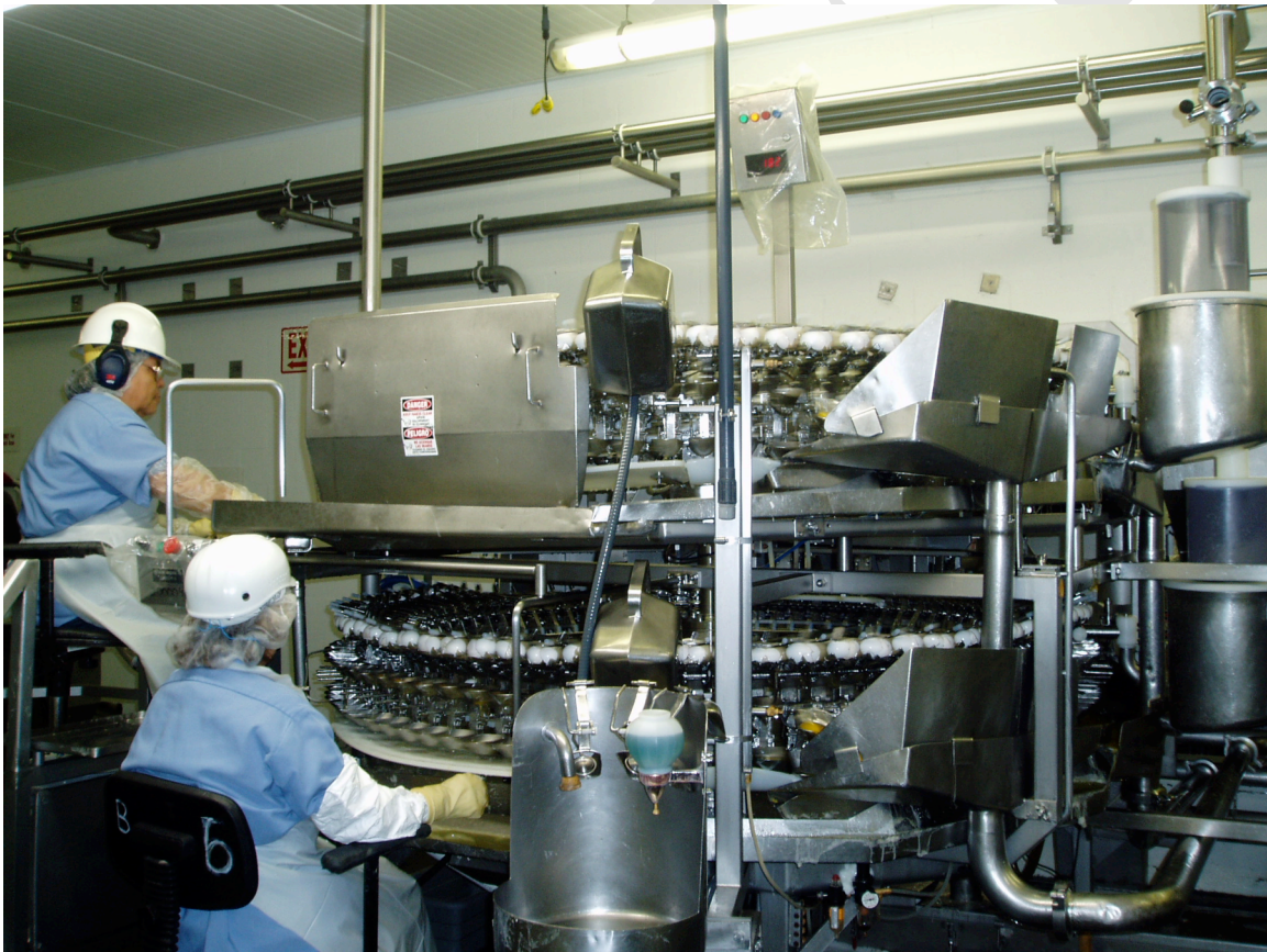
Figure 2. Photo of a high-speed egg breaker with inspectors.
